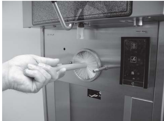
Figure 24. Cleaning Freezer Barrel
