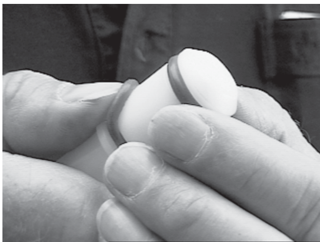
Figure 23. Removing "O" Ring
