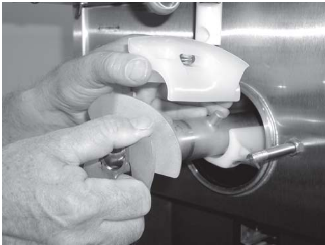
Figure 22. Auger Shaft Removal
